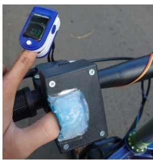
Figure 7. Testing the MAX30102 Sensor and Validator by Riding a Treadmill Bike
